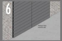
When butting two boards together, you should left minimum 4mm gap between the boards. To prevent moisture, a minimum of 20 mm of space should be left from the ground and the bottom edge of the boards. Between the boards edges and solid walls/objects minimum 8mm gap needs to be left. Not leaving the
